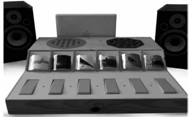
Fig. 5. The instrument "Sound in Hands" designed by McAdams and Bigand in 1993, composed of two speakers, a response platform and a computer.
