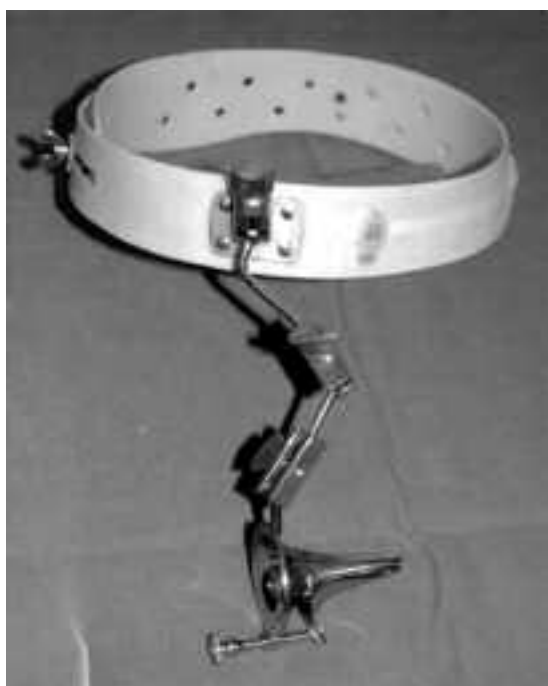
Fig. 1. Custom self-retaining nasal speculum allows surgeon to have both hands free, making laser treatment easier to perform and in less time.
